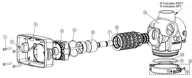
Install V3672 upper diffuser (not shown) when using the 6" Flange Base (V3090)
